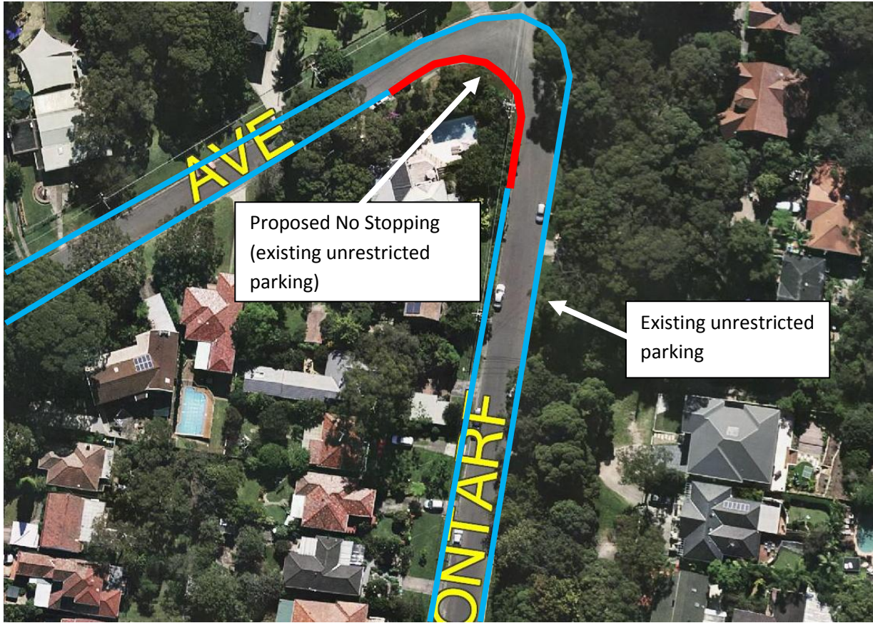
Figure 2: Proposed installation of No Stopping restrictions at Alto Avenue and Clontarf Street
