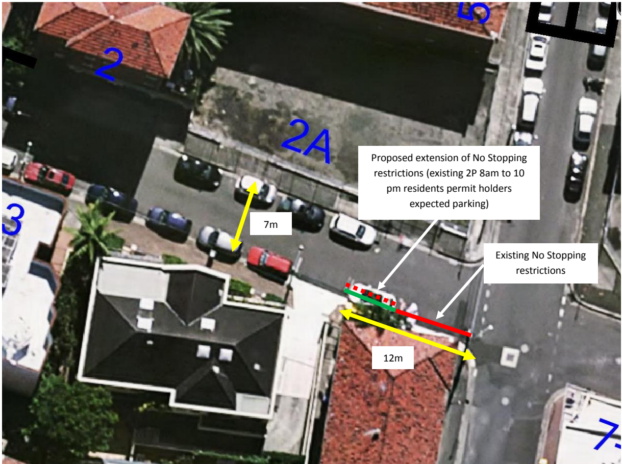
Figure 1: Proposed removal of one on street parking space and introduction of No Stopping restrictions
