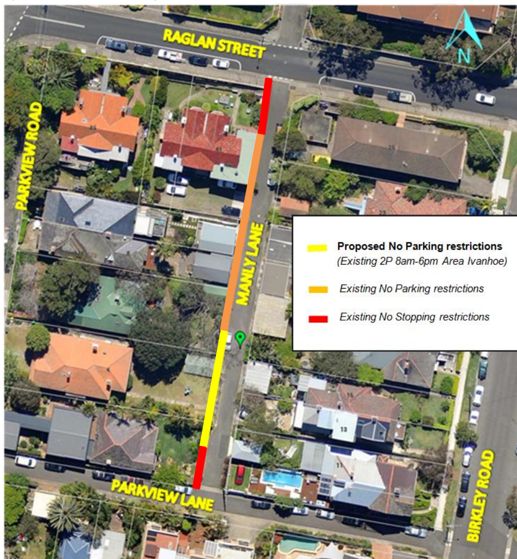
Figure 4: Proposal to extend No Parking restrictions on the western side of Manly Lane.
