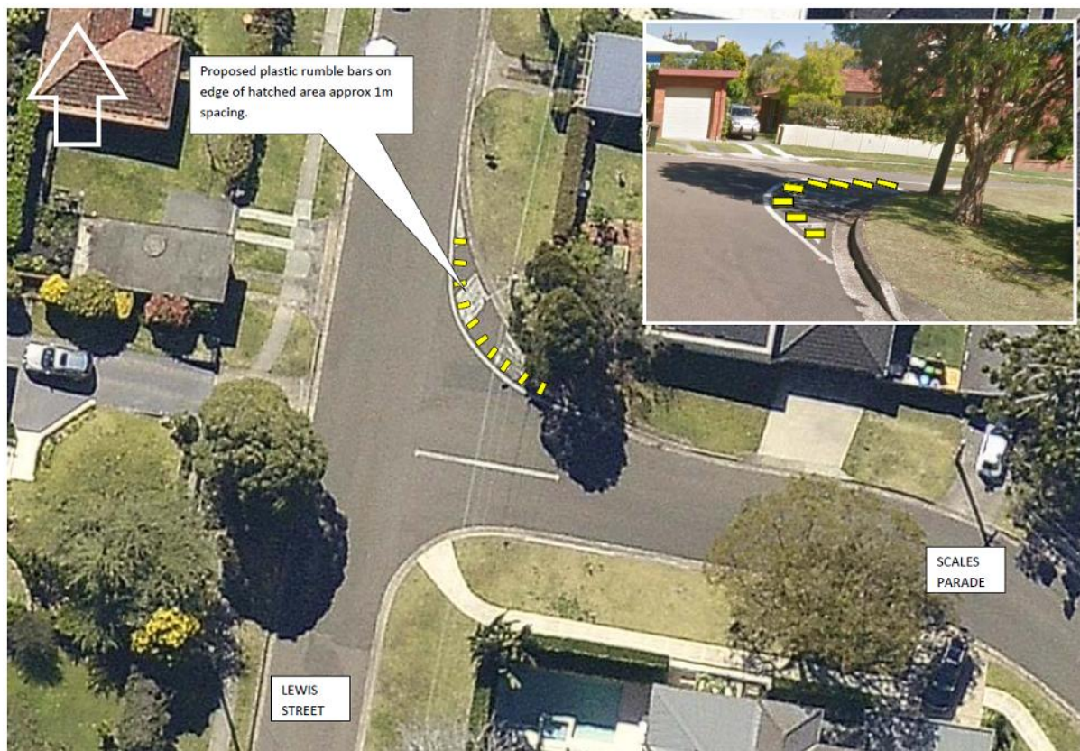
Figure 9: Proposal to install rumble bars on the north eastern corner of Scales Parade / Lewis Street intersection.
