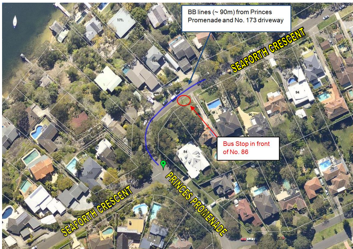
Figure11: Proposed double barrier centrelines between Princes Promenade to No. 173's driveway, approximately 90 metres.
