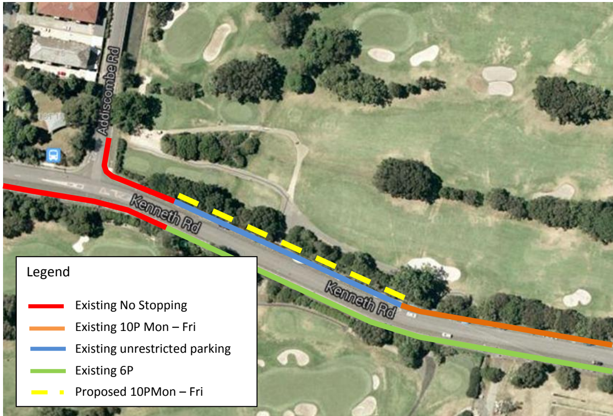
Figure 17: Site location and existing parking restrictions at Kenneth Road, Balgowlah
