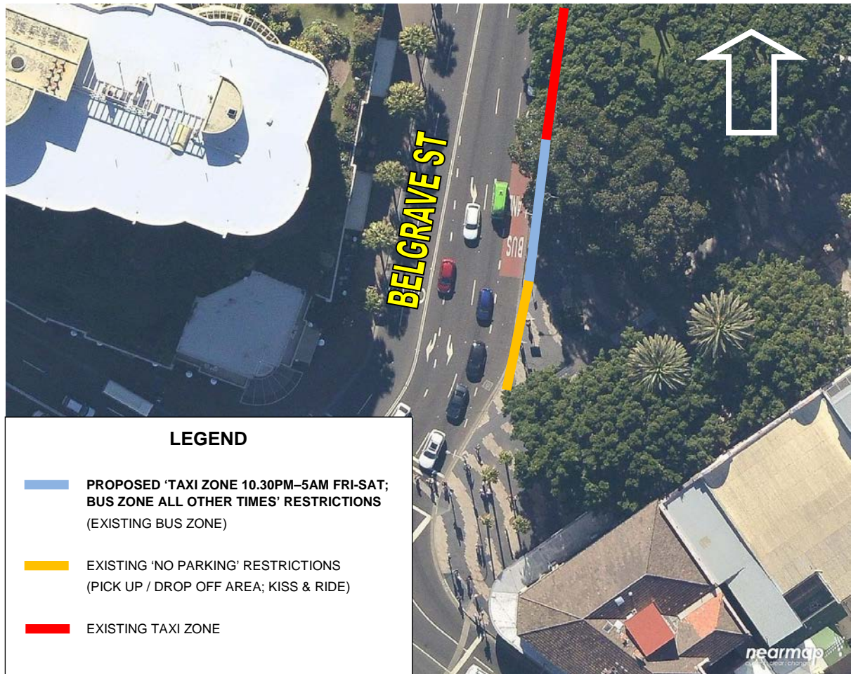
Figure 3: Aerial of Belgrave Street with proposal to amend the existing bus zone
