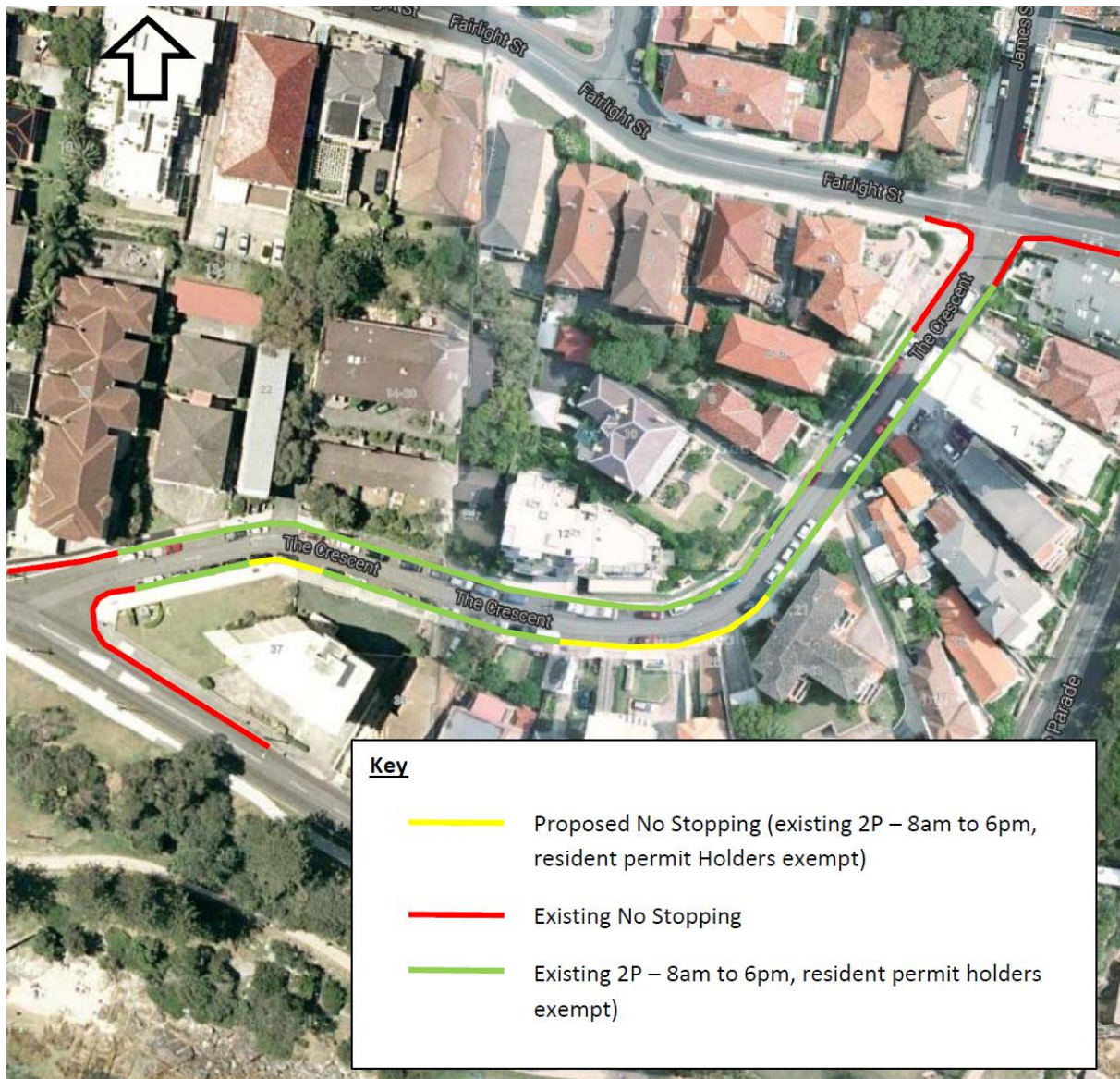
Figure 9: Proposed No Stopping restrictions on southern side of The Crescent between No. 21 to No. 31
