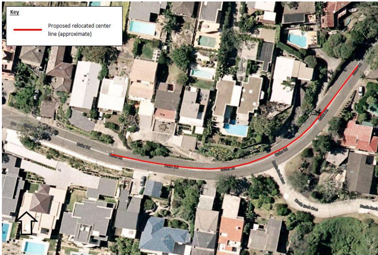
Figure 10: Proposal to realign the centre line in Cutler Road between No. 59 & No. 75 by 400mm north
