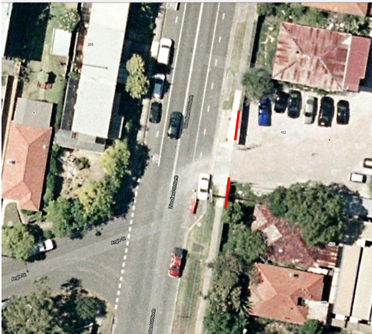
Figure 1 - Introduction of 10m No Stopping restriction – Sylvan Avenue, Balgowlah
