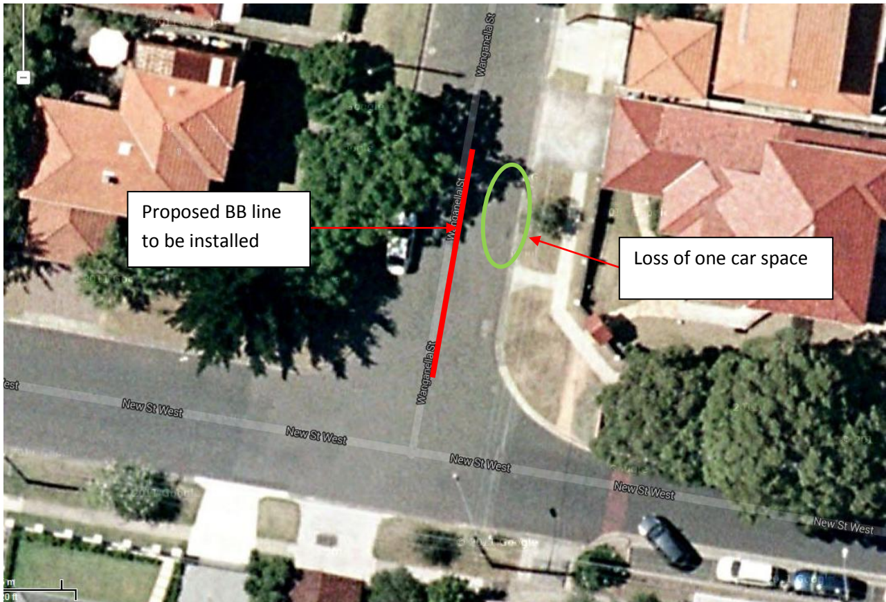
Figure 1: Proposed BB line – Wanganella Street at the intersection with New Street, Balgowlah
