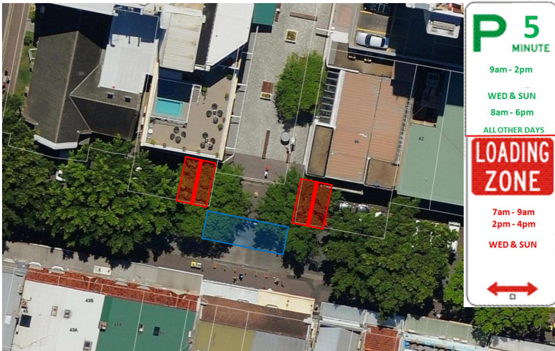
Figure 11: Proposed 4 additional P5 min/Loading zone parking bays on either side of existing P5 min bay.
