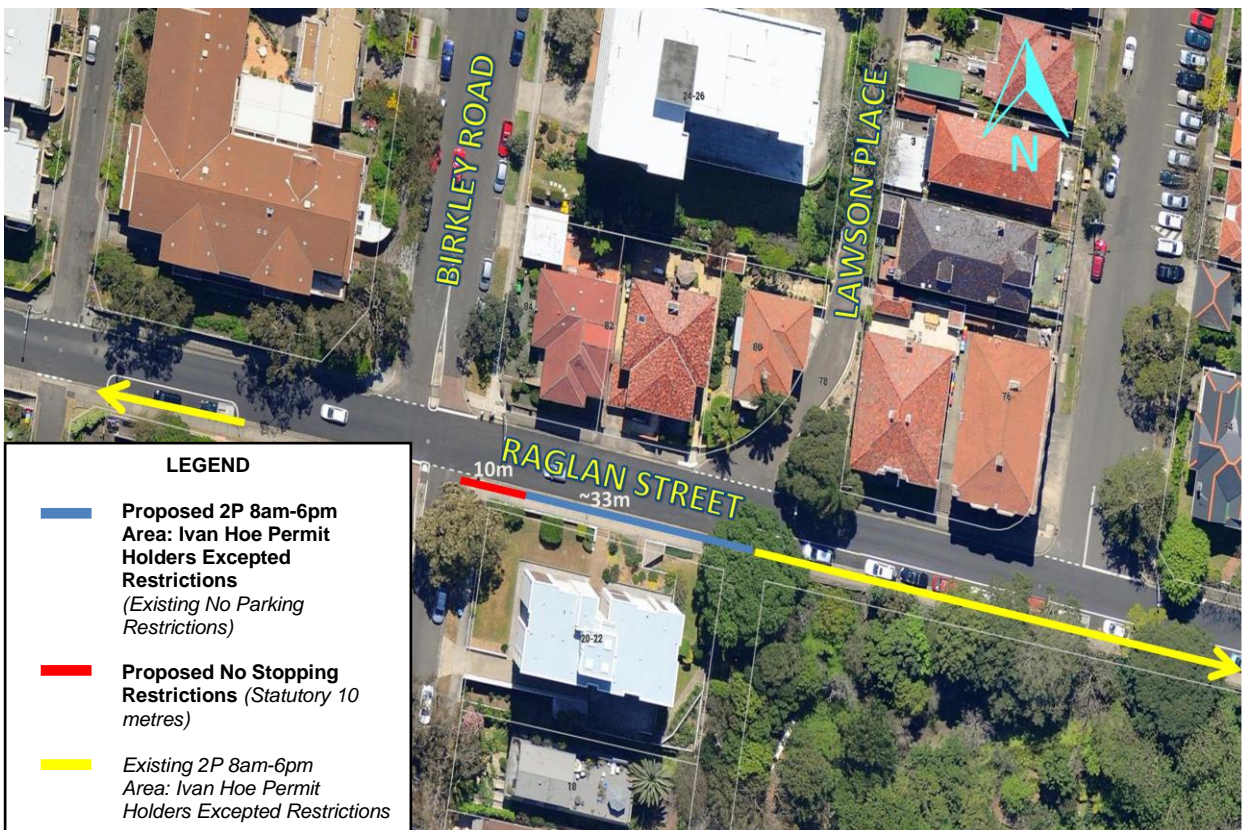
Figure 6: Proposed 2P Ivan Hoe Park Residential Parking Scheme to replace No Parking restrictions.
